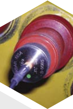
Ultrasonic measurement of sub sea flange
