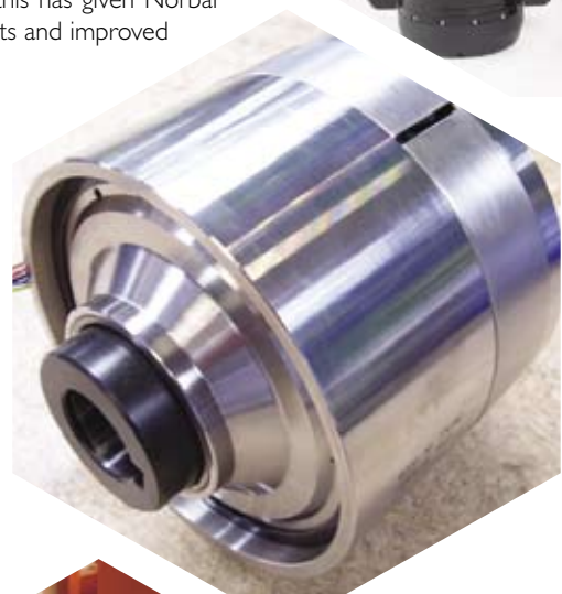
Pipe clamp tool showing manipulating handle, Locking pin, reaction plate and pressure compensation. Input drive will be from an API Class 4 17D tool.
